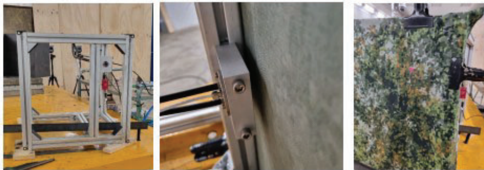
Figure 4. View of the sample rack and heat flux sensor position in relation to sample. The sensor was aligned to the centre of the laser spot.
