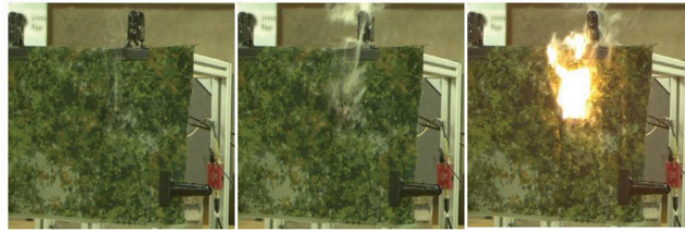
Figure 8. NFP Green with a power setting of 913 W and a spot diameter of 8 cm (artillery scenario). Figures from left to right show smoke formation after 1.5 s, start of burn after 2.3 s and fire after 2.4 s.
