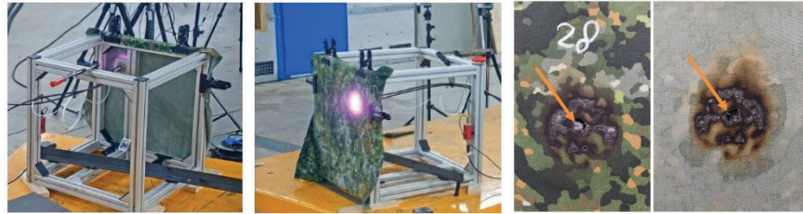
Figure 5. Left and middle: NFP Green non FR during laser irradiation (back and front view), settings: 155W, 8 cm spot diameter. Right: results after 15 seconds (perforation).
