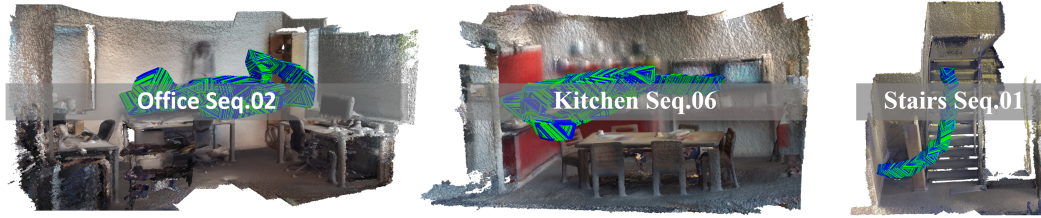
Figure 4: The visualization results of camera pose on 7 Scenes. In each scene, the green and blue poses denote the ground truth and prediction respectively.
