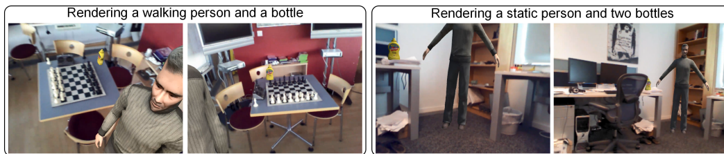
Figure 5: AR effect on the Chess and Office scene of 7 Scenes. We render a virtual walking person and a bottle onto the Chess scene, and two virtual bottles and a static person onto the Office scene based on the predicted camera pose of our framework.
