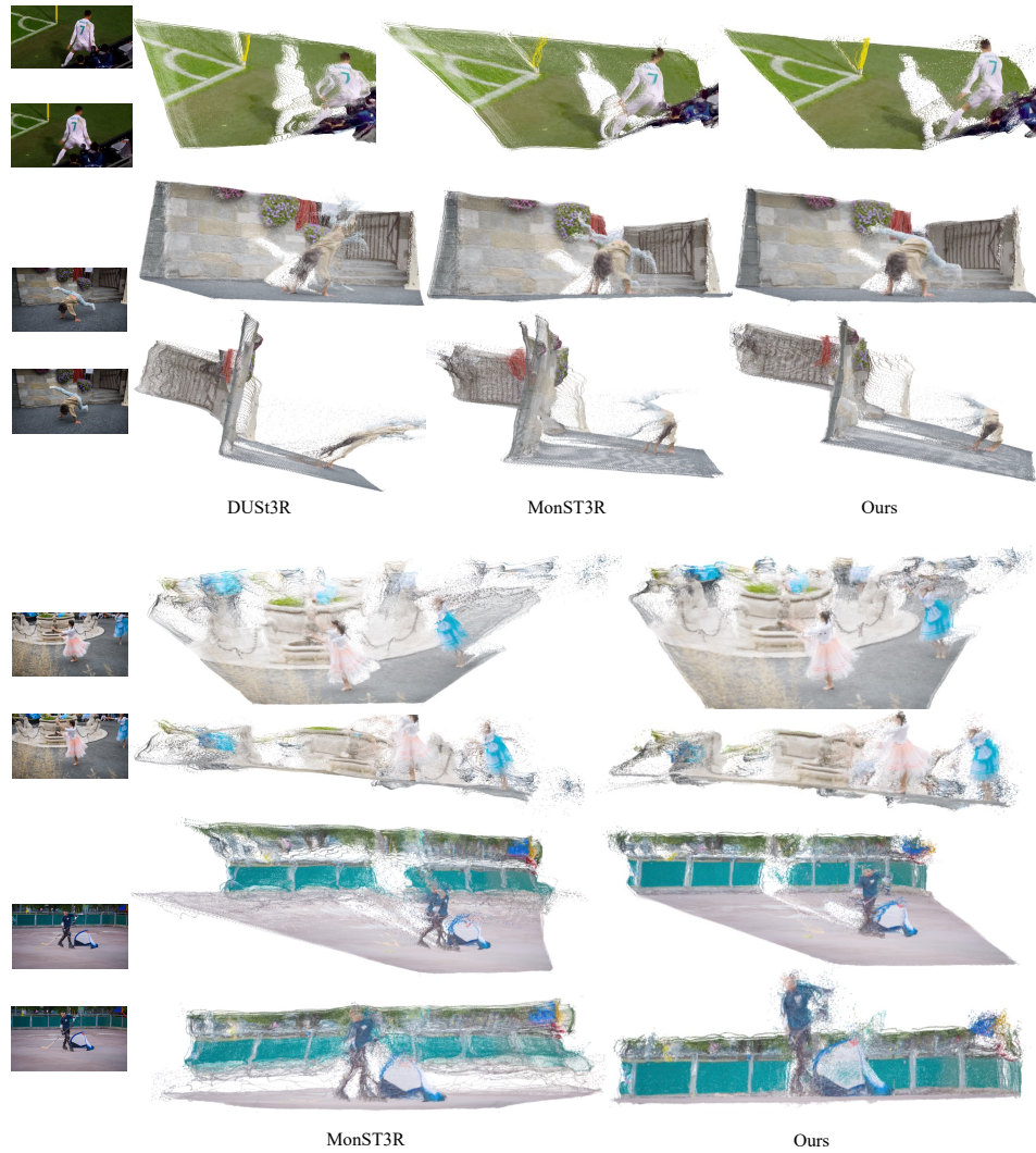
Figure 5: Pointmap reconstruction. We qualitatively compare the 3D pointmap of D^2USt3R against other pointmap regression models [44, 51]. All visualizations presents per-pixel pointmaps without applying confidence thresholding. It is notable that both DUST3R [44] and MonST3R [51] struggle to accurately reconstruct scenes that include dynamic object. We find that inaccurately established correspondence fields between dynamic regions negatively affect the overall reconstruction performance.
