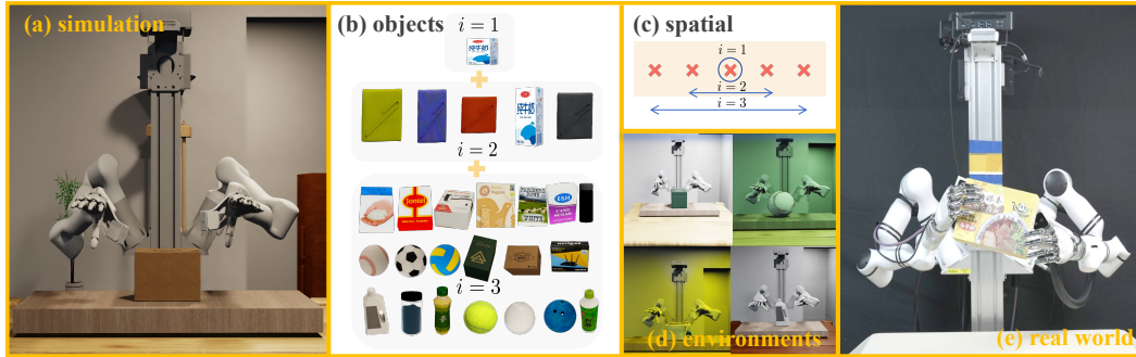
Figure 3: Experiment Setup. Taking the dual-arm robot system as an example, (a) Our simulation environment. (b) Object diversity expansion across iterations, progressing from a single object ( i=1 ) to geometrically similar objects ( i=2 ) and diverse geometries and physical properties objects ( i=3 ). (c) Spatial diversity, showing the spatial arrangements. (d) Environment diversity, including variations in lighting conditions and tabletop appearances. (e) Real-world environment.
