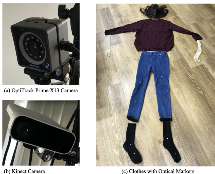
Figure 4: Devices and marker-fitted clothing used for data collection.
