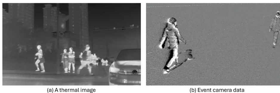
Figure 5: Pedestrians captured by thermal and event cameras. These data can still pose privacy risks. (a) A thermal image containing pedestrians (image taken from the FMB dataset Liu et al. [2023a]). (b) Pedestrians captured by a Prophesee event camera (image taken from Moore [2020]).
