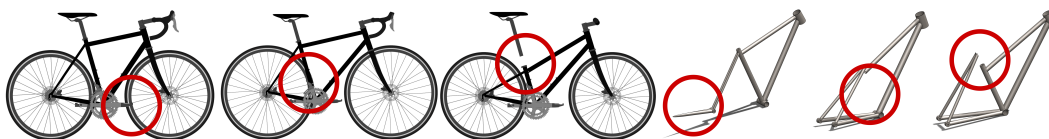
Figure 10: BikeBench features numerous closed-form constraint checks to identify common geometric infeasibilities such as disconnected or colliding components (left 3). Less common infeasibilities in frame geometry are flagged if the design causes errors during 3D reconstruction (right 3).
