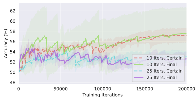
Figure 18: Test accuracies for LSTM baselines, trained with either the certainty-based loss or the cross-entropy loss at the final internal tick. Both loss functions lead to unstable learning.
