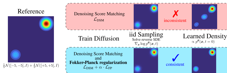
Figure 1: Training diffusion models on a 2D toy example reveals inconsistencies. While classical iid diffusion sampling (i.e., denoising) correctly reproduces both modes, evaluating the score at t = 0 to estimate the unnormalized density yields a third mode and an incorrect mass distribution. Such a diffusion model would produce incorrect dynamics while producing correct samples. A model trained with Fokker–Planck regularization is self-consistent, and aligns the learned score at t = 0 with the distribution recovered by diffusion sampling.
