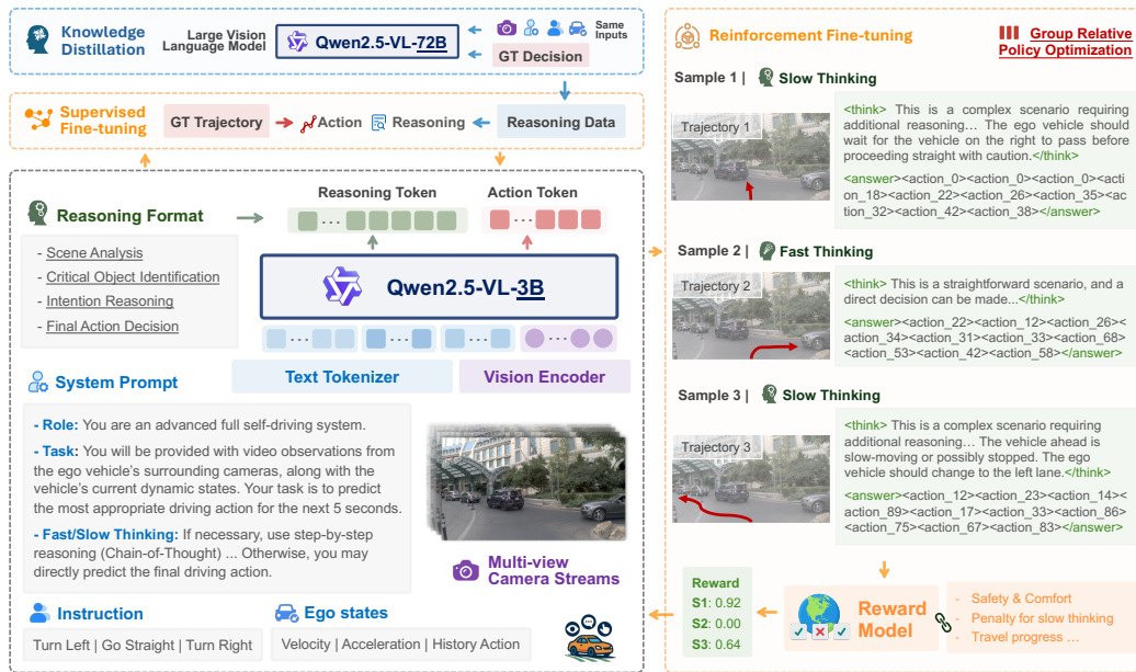
Figure 3: Overview of the AutoVLA model and its training process. A pretrained small VLM is used as the backbone of AutoVLA. The model receives multi-view camera streams, system prompts, driving instructions, and vehicle status as input, and outputs textual reasoning and physical action tokens. In SFT, a large VLM model with strong visual understanding capabilities is employed to collect reasoning data, which is used alongside trajectory data in SFT for training the AutoVLA model. In RFT, we utilize GRPO to train the model for improved alignment with verified reward functions, while enabling adaptive reasoning by penalizing excessive reasoning.
