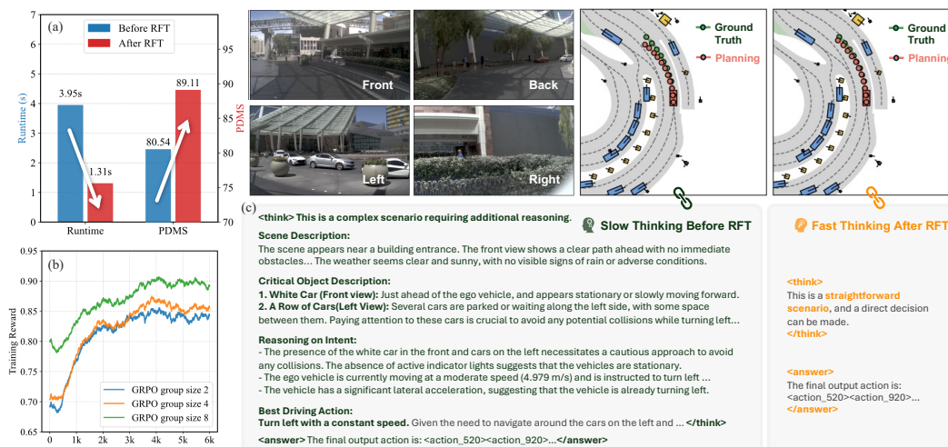
Figure 5: Reinforcement fine-tuning results on the nuPlan dataset. (a) Comparison of PDMS and runtime before and after RFT; (b) Training reward curves for different GRPO group sample sizes; (c) Qualitative comparison of planning and reasoning performance before and after RFT.
