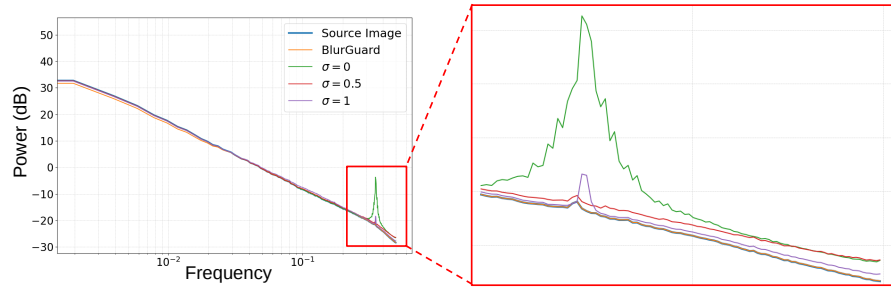
Figure 7: Comparison of the Radially-Averaged Power Spectral Density (RAPSD) of image protections using constant Gaussian blur intensity \sigma . The deviation in high-frequency bands (right side of the plot) often corresponds to the vulnerability against noise purification.
