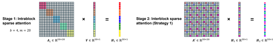
Figure 2: DuSA performs intrablock sparse attention within each block to obtain local inductive biases in Stage 1. DuSA performs interblock sparse attention to obtain global information in Stage 2. Here the blockify strategy is Strategy 1 in Remark 1. The different colors in attention matrices ( A_1 and A_2 = A' ) denote the different blocks. The color changes between V and H_1 and between H_1 and H_2 denote the information aggregation process.
