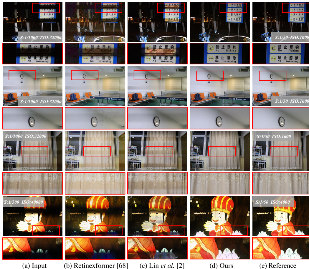
Figure 6: Visual results of flicker removal on the static test data. Our results are obtained by training the Restormer on our dataset. It demonstrates the best performance across diverse flickering scenes.
