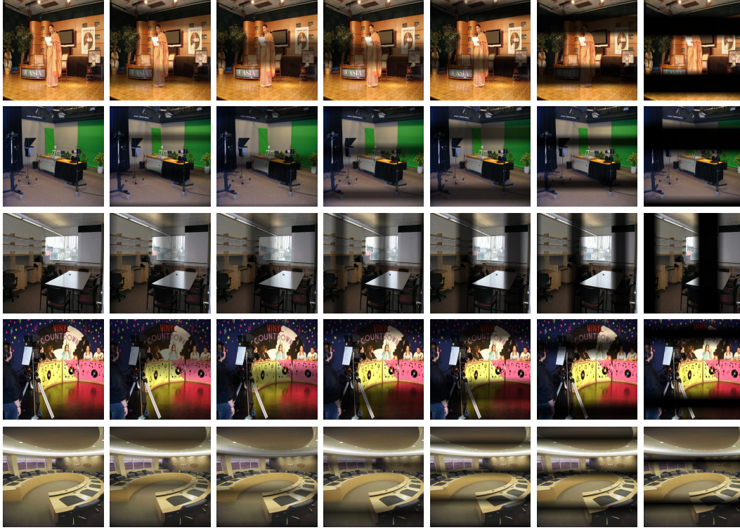
Figure 3: Flicker synthesis results based on the proposed Retinex-based method. Background images are sourced from the indoorCVPR dataset [63]. A pre-training is conducted using the synthetic data, providing a strong initialization for subsequent training on real data.
