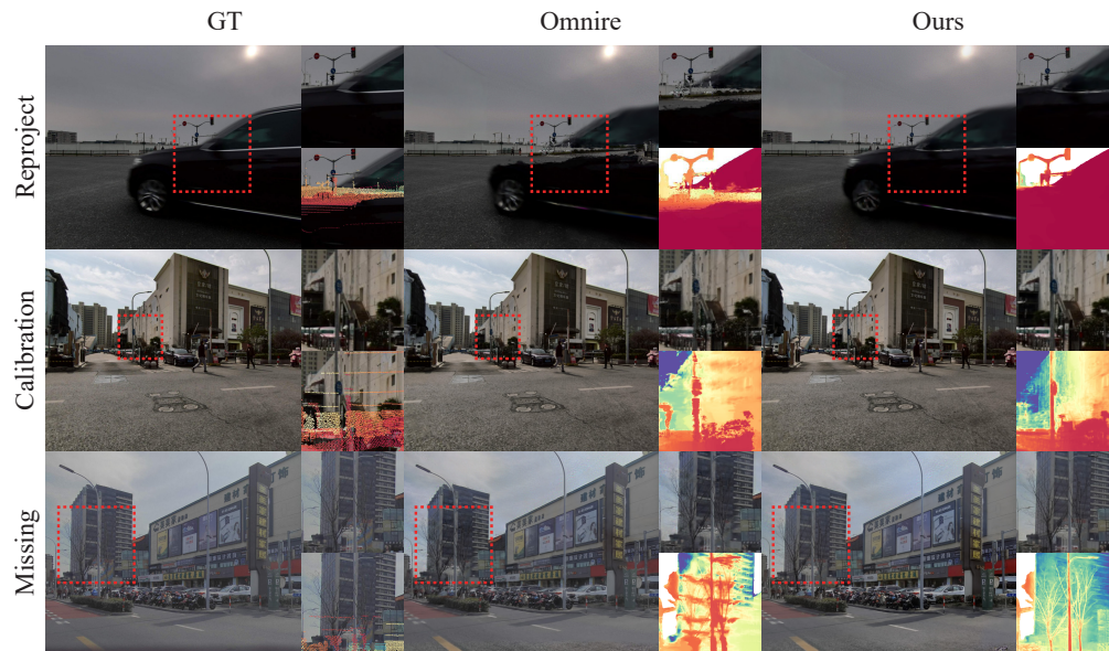
Figure 1: Examples of common LiDAR acquisition issues: a) reprojection error, b) calibration misalignments, and c) LiDAR missing problem. OmniRe [1] yields poor performance in both image reconstruction and depth estimation when using these inaccurate LiDAR measurements.
