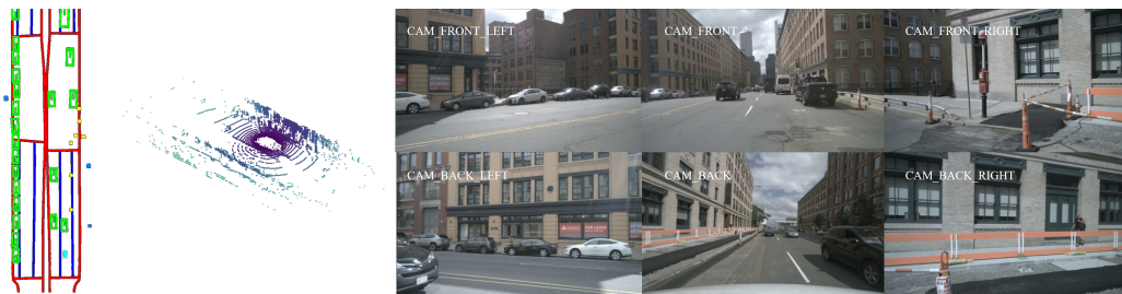
Figure 12: Joint generation of LiDAR and multi-view video. Our method generates spatially aligned LiDAR and camera views conditioned on a shared straight street layout.
