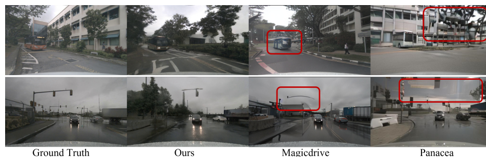
Figure 10: Qualitative comparison of video generation quality. Our method (second column) preserves accurate layout, object shapes, and background integrity. MagicDrive (third column) shows vehicle distortion and broken structures. Panacea (fourth column) often suffers from hallucinated textures and geometric misalignment.
