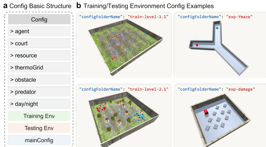
Figure 9: Overview of the configuration system of EVAAA. (a) Modular config hierarchy, organized by components such as agent, court, resource, and obstacle. (b) Example instantiations for training (e.g., train-level-1.1, train-level-2.1) and testing (e.g., exp-Ymaze, exp-damage) via the configFolderName parameter.
