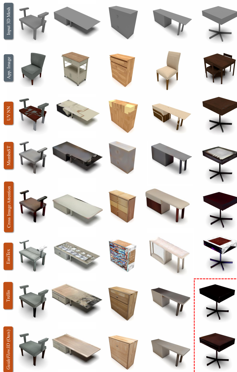
Figure 12: Qualitative Comparisons showing results using image condition with \mathcal{L}_{\text{appearance}} . We show 5 examples (one per column) and the results for all methods. UV Nearest Neighbor (UV NN) often misplaces textures across parts but performs better with uniform materials. MambaST, Cross Image Attention, and EasiTex blend or oversmooth textures, while Trellis improves realism yet lacks geometric grounding. GuideFlow3D achieves semantically and structurally consistent transfers, accurately mapping materials like upholstery and wood. Column 5 illustrates a failure case for all methods, though UV NN yields the most visually coherent result and our interleaved guidance scheme cannot recover from the black output produced by Trellis.
