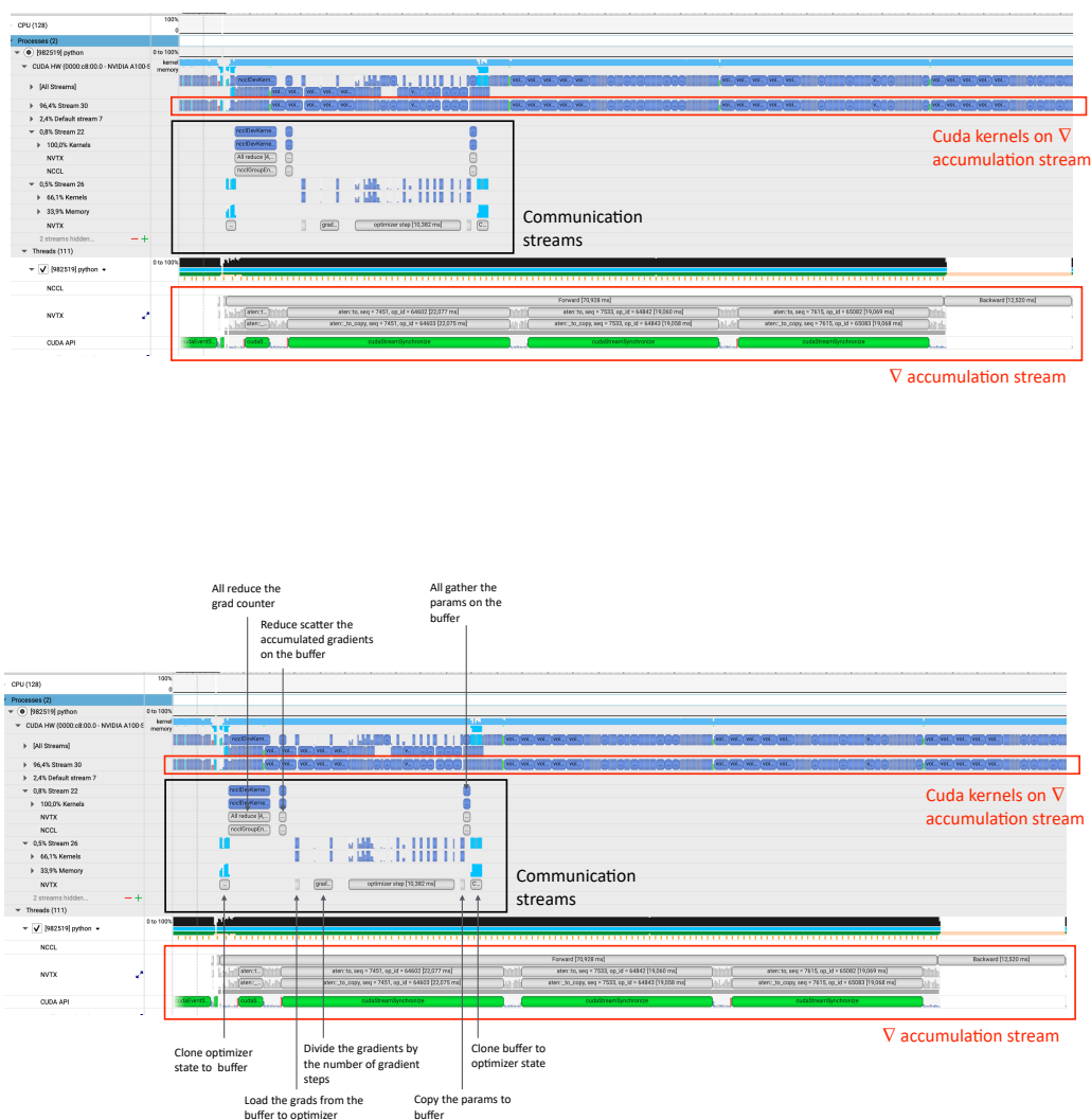
Figure 13: Nsight system profile of our implementation of ACCO: our two streams do run in parallel. In this Figure, the computation take more time than the communication because we only profiled small scale experiments with 8 workers, and small number of parameters (36M as we profiled on our TinyStories [16] setting). This changes when using larger models and more workers, as seen in 4.1.
