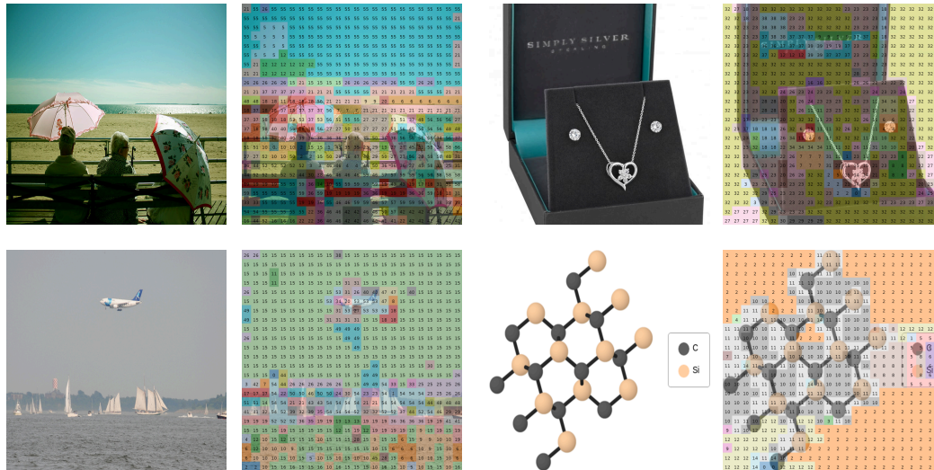
Figure 7: Visualization of merged patch tokens by DYMU. Patches with the same color are merged into a single token, and the number inside each patch indicates the final merged token index. We find that the merging adapts to the complexity of the regions: simpler regions, such as the sky or a white background, tend to be merged more, while complex regions preserve a larger number of unique tokens.
