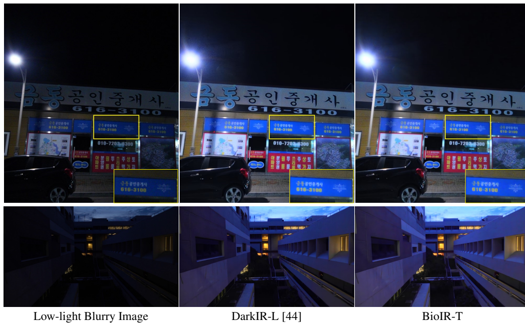
Figure 10: Generalization evaluation by directly applying the model pretrained on LOLBlur [43] to real-world night blurry images. The top example is from the RealBlur [90] dataset, while the bottom example is captured in an uncontrolled real-world setting. Our model more effectively restores both text details and overall brightness.
