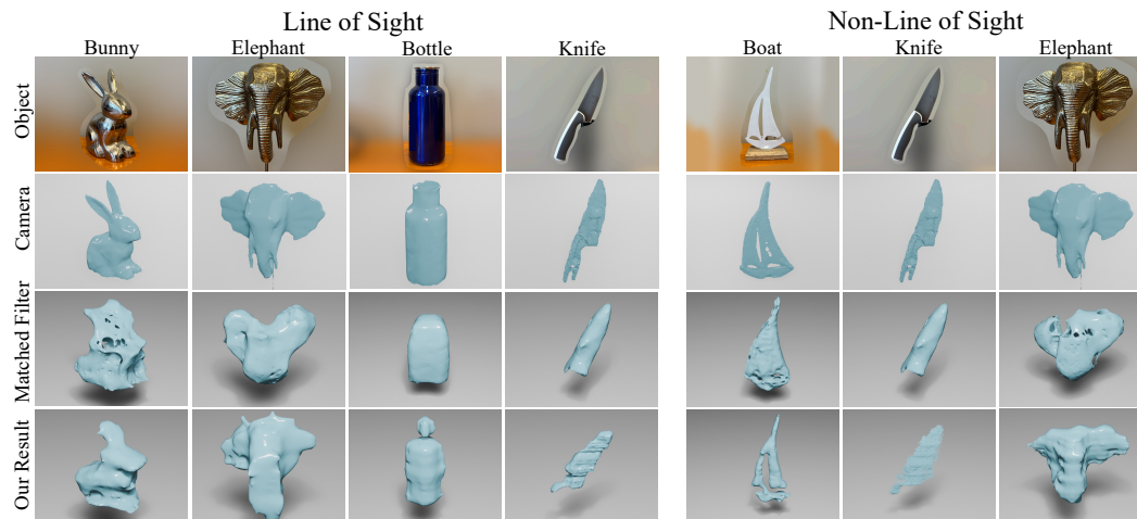
Figure 6: Left: Experimental results of objects with nothing between the radar and the object. Right: Results when the object is occluded from the radar. The camera scan done in line of sight.
