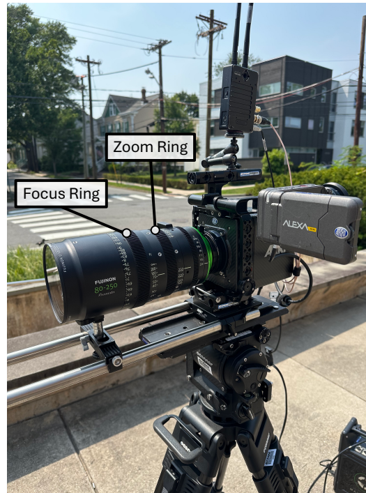
Figure N: Diagram of the premista80 lens used. Rotating its zoom and focus rings shifts internal lens groups, changing the camera intrinsics.
