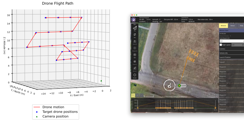
Figure G: A visualization of an example 3D drone path. The camera space coordinates are shown on the left, and the corresponding QGroundControl mission is shown on the right.
