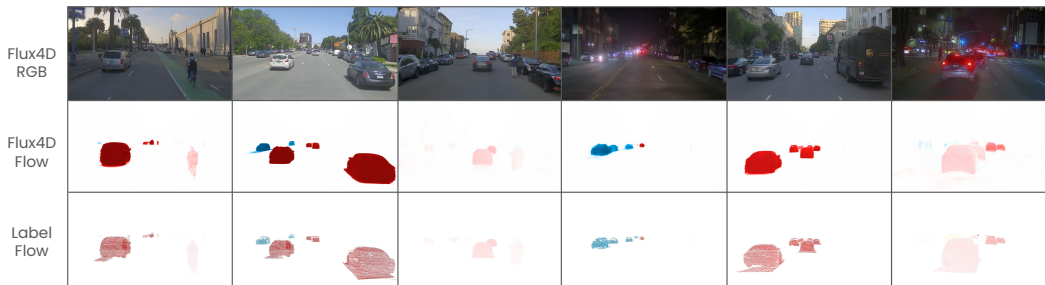
Figure 6: High-fidelity flow and RGB reconstruction . Flux4D not only provides photorealistic reconstruction of the dynamic scene but also estimates actors’ motion flow with high precision.
