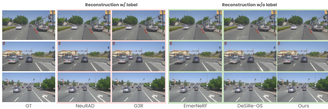
Figure 4: NVS on longer-horizon logs. Qualitative comparison shows that our method outperforms SoTA unsupervised baselines, by maintaining better estimation of actor movements in longer horizon. We shrink the gap in quality to supervised methods.
