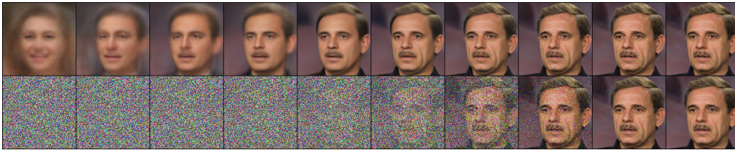
Figure 7: Sampling trajectory for greedy (midpoint) solving the HDR inverse problem. Top row is midpoint estimate and the bottom row is x_t .
