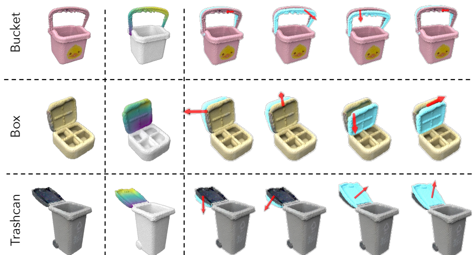
Figure 6: Real-world visualization of the motion prior network on the AKB-48 [26] dataset. We used our trained motion prior model in PartNet-Mobility to estimate normal motion for the real-world scanned objects from the AKB-48 dataset. For each row, we show the input point cloud, the movability score map, and four sampled action-motion pairs, respectively. The sampling of action-motion pair is performed based on the normalized scores. Red arrows indicate the input actions, and the anticipated motions are shown in cyan.
