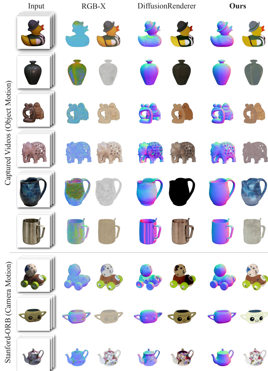
Figure 8: Outputs from captured videos of real world objects. Our model effectively uses differential motion to produce higher-quality estimations of shape and albedo compared to RGB-X and DiffusionRenderer.
