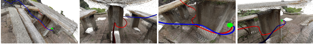
Figure 11: VGER enables smooth collision-free motion. Here, two trajectories (red and blue) warp over benches and around the leg of the table to reach the goal (green).
