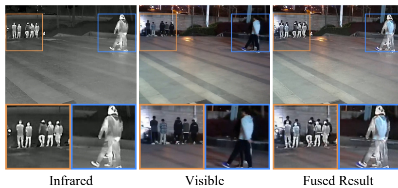
Figure 18: Artifacts in fused video caused by misaligned input frames.
