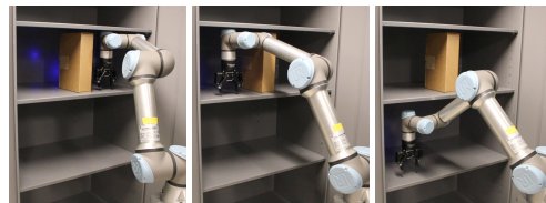
Figure 3: ACQL policies trained with safety constraints based a cabinet’s geometry can be successfully deployed for a UR5e manipulator operating in the real cabinet environment.
