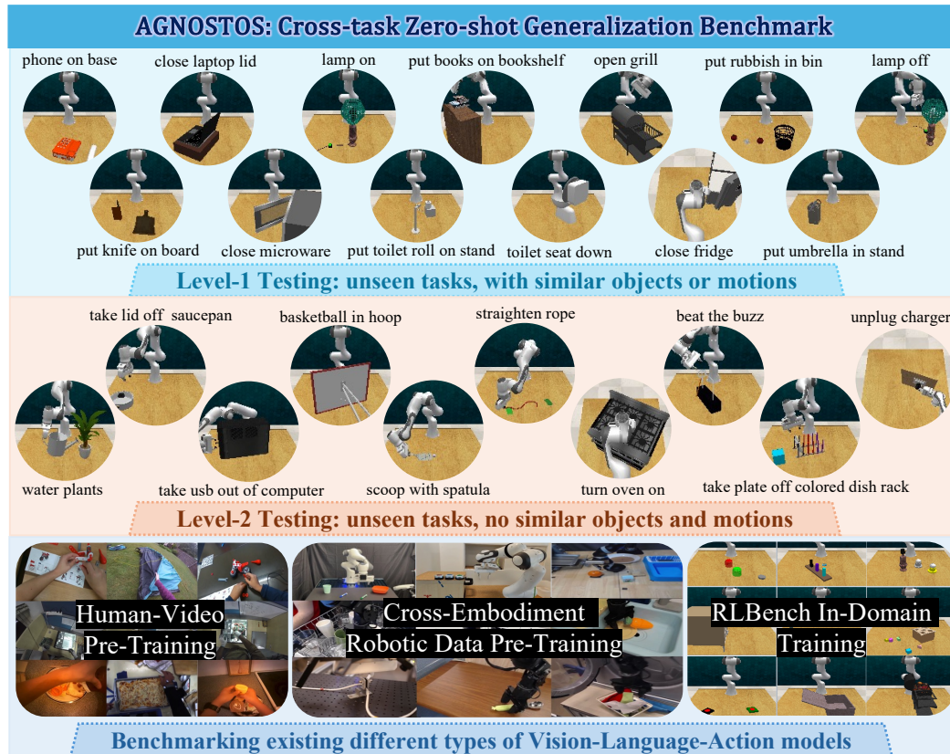
Figure 1: The proposed AGNOSTOS benchmark evaluates zero-shot cross-task generalization through two difficulty levels. Level-1 testing involves 13 unseen tasks sharing partial similarity (objects or motions) with seen tasks. Level-2 testing has 10 unseen tasks from entirely novel scenarios, requiring stronger generalization capabilities. We systematically assess three broad categories of vision-language-action models, revealing critical limits in their ability to adapt to unseen tasks.
