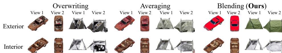
Figure 4: Analysis on UV texture merging techniques. Compared to naive approaches, our blending strategy preserves clear structural boundaries and significantly improves texture quality.
