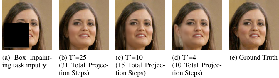
Figure 6: We show how the results change as we decrease the number of denoising steps T' . Notably, we still produce reasonable results with only T' = 4 denoising steps and a corresponding 10 total projection steps, for a total of 14 Neural Function Evaluations (NFEs) and < 1 second inference.
