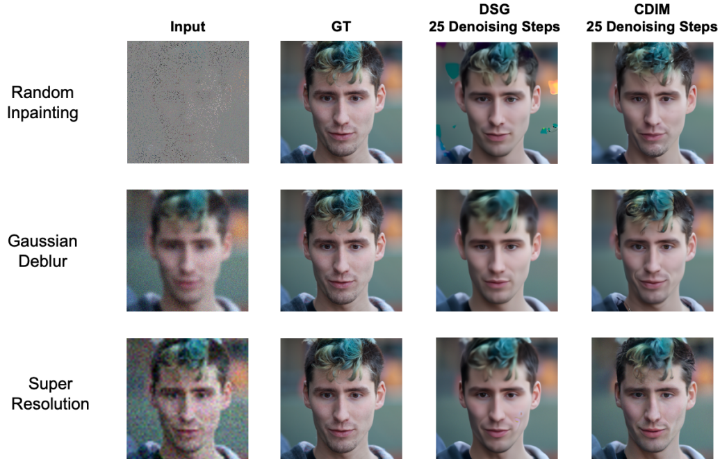
Figure 10: A comparison between CDIM and DSG [28] when both algorithms use 25 DDIM denoising steps. Notice the artifacts in the DSG random inpainting.
