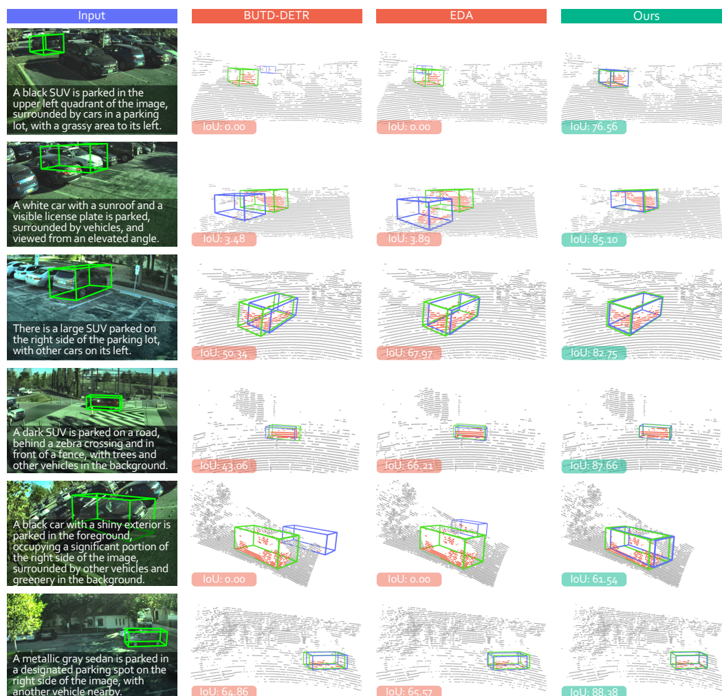
Figure 15: Additional qualitative comparisons of single-object 3D grounding on the Drone platform from the 3ED dataset. The data shown include the RGB frames, the LiDAR point clouds, and the associated referring expressions. The ground truth and predicted boxes are shown in green and blue, respectively. Best viewed in colors and zoomed in for more details.
