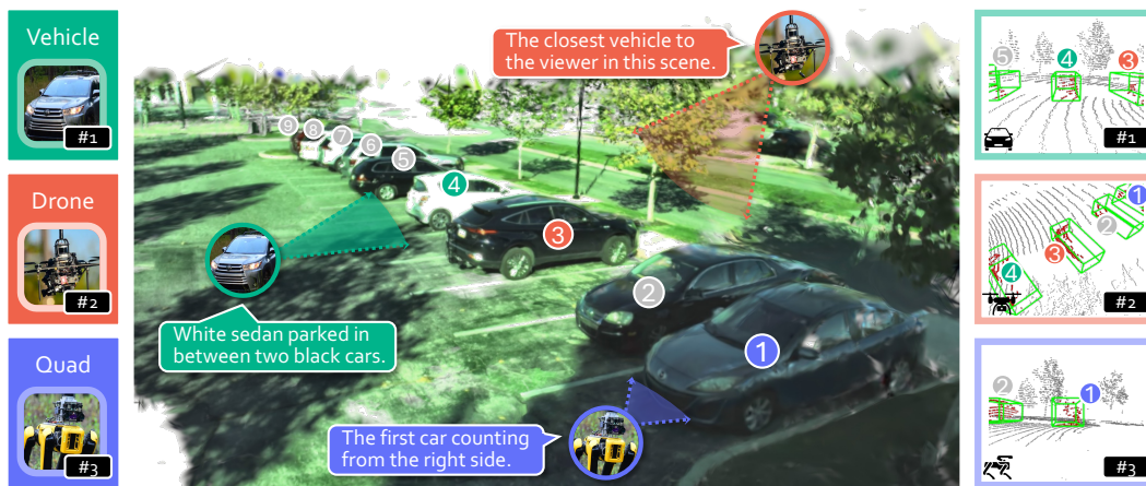
Figure 1: Multi-modal, multi-platform 3D grounding from 3EED. Given a scene and a structured natural language expression, the task is to localize the referred object in 3D space. Our dataset captures diverse embodied viewpoints from Vehicle, Drone, Quadrupeid platforms, presenting unique challenges in spatial reasoning, scene analysis, and cross-platform 3D generalization.
