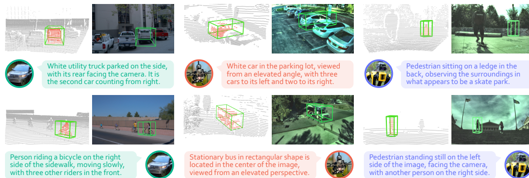
Figure 3: Examples of multi-platform 3D grounding from the 3EED dataset. There are clear discrepancies across both sensory data (2D & 3D) and referring expressions from the Vehicle, Drone, and Quadrupe platforms. For additional examples, kindly refer to the Appendix.
