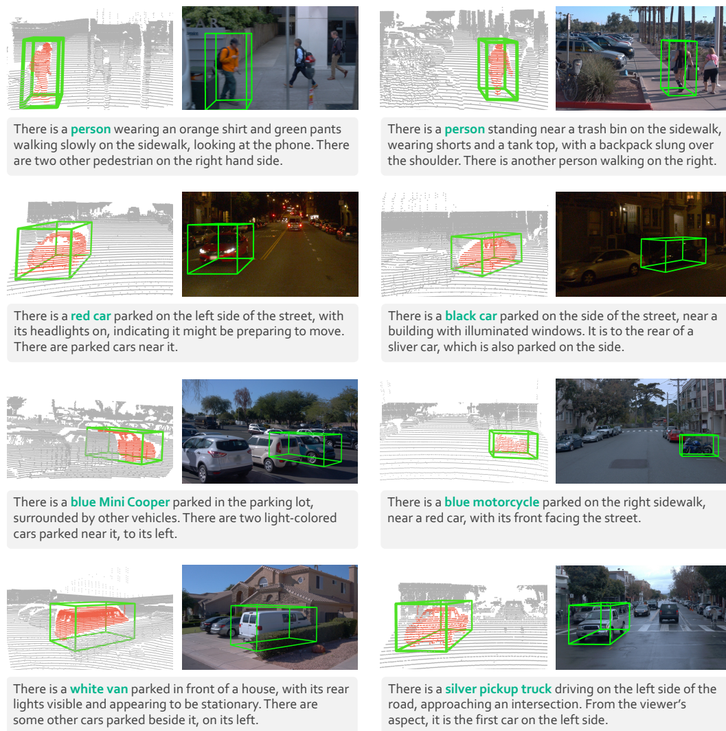
Figure 9: Additional examples of 3D grounding from the Vehicle platform in 3ED dataset. The data shown include the LiDAR point clouds, the RGB frames, and the associated referring expressions. Best viewed in colors and zoomed in for more details.
