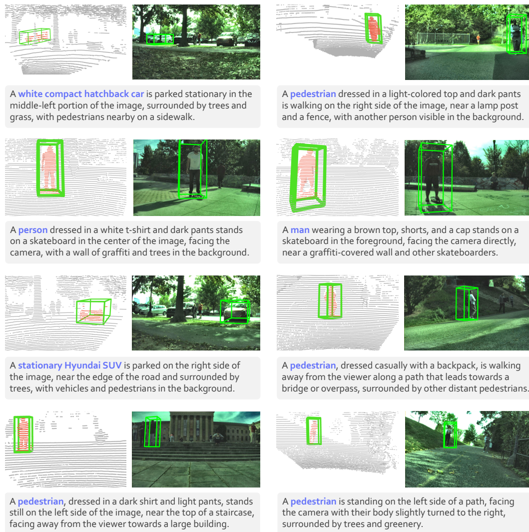
Figure 11: Additional examples of 3D grounding from the Quadruped platform in 3EED dataset. The data shown include the LiDAR point clouds, the RGB frames, and the associated referring expressions. Best viewed in colors and zoomed in for more details.
