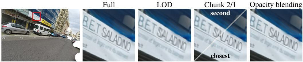
Figure 7: Ablation study. We compare the full representation (without LOD), full LOD, rendering from closest and second closest LOD chunks, and opacity blending.
