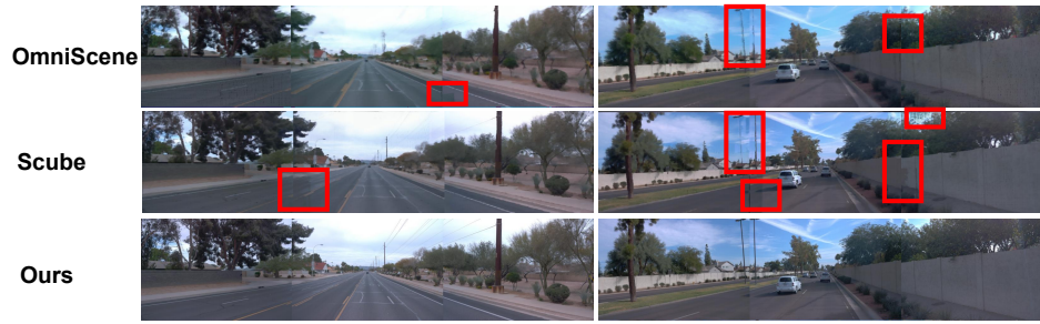
Figure 4: Reconstruction quantitative comparison. The red box indicates the presence of artifacts in the overlap area of multi-view images, due to Gaussian prediction at per-pixel level ( zoom in for the best view. )
