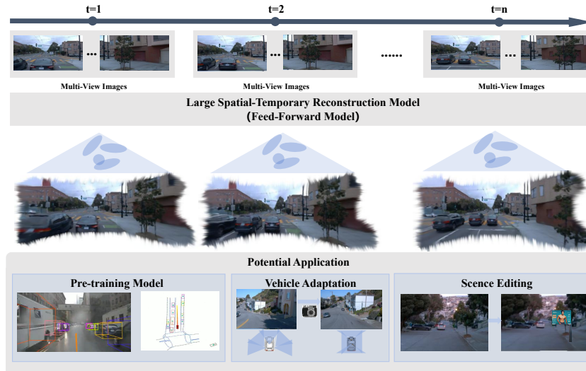
Figure 1: Leveraging temporal multi-view images, the Large 4D Gaussian Reconstruction Model (DrivingRecon) can predict 4D driving scenes. DrivingRecon serves as a pre-trained model that effectively captures geometric and motion information. Additionally, DrivingRecon can synthesize novel views based on specific camera parameters, ensuring adaptability to various vehicle models. DrivingRecon further facilitates editing of designated 4D scenes.
