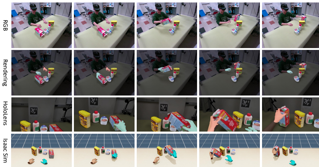
Figure 1: Sample capture from HO-Cap. From top to bottom: RGB frames, overlaid renderings of 3D shape and pose for hands and objects in third-person and egocentric views, and renderings of the capture within a virtualized scene in the NVIDIA Isaac Sim simulator.
