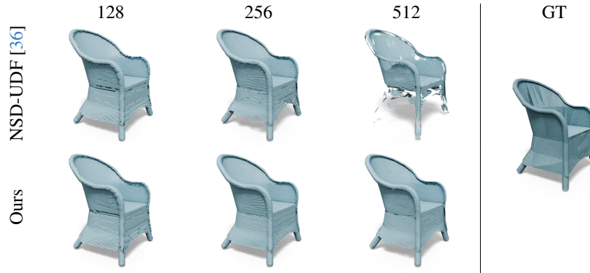
Figure A.1: Meshing at different resolutions, additional examples. While NSD-UDF [36] retrieves most of the surface well at a low resolution, it struggles at higher ones. In contrast, our method, recovers the surface well at all resolutions. We use Marching Cubes with both methods.
