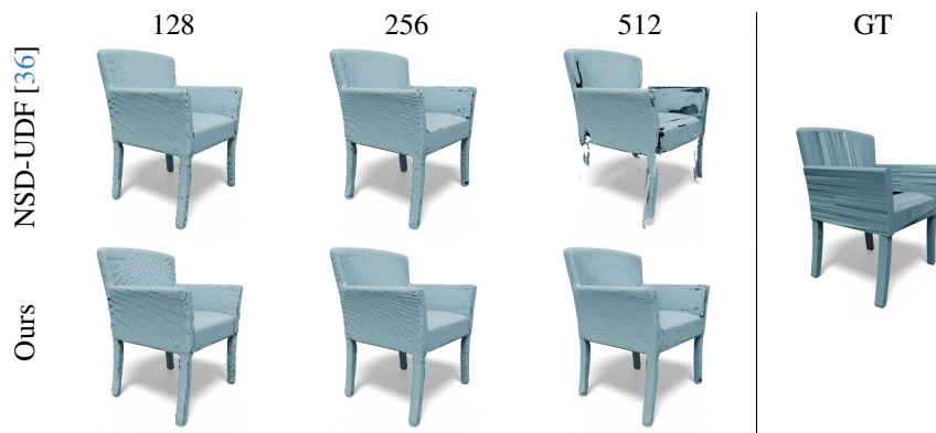
Figure 5: Meshing at different resolutions. While NSD-UDF [36] retrieves most of the surface well at a low resolution, it struggles at higher ones. In contrast, our method, recovers the surface well at all resolutions. We use Marching Cubes with both methods.
