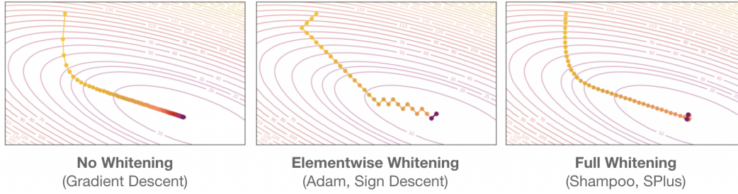
Figure 1: Whitening normalizes gradients to have uniform magnitude along each axis of descent. This decouples the updates from gradient magnitude. Elementwise whitening imposes an independent axis per dimension, whereas full whitening uses the axes that maximally explain gradient covariance.
